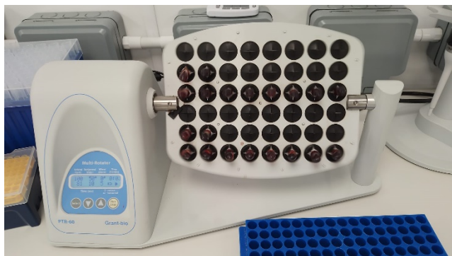
(fig.2) The samples were spun in a rotator. This helps in the immersion of the cell suspension.
